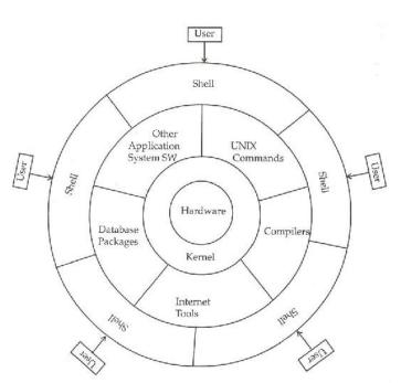
Fig 1.1: Structure of UNIX Operating System
