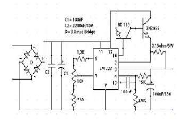
Let , Error amplifier controls the series pass transistor Q2 which acts as a variable resistor. The series pass transistor is small power transistor having about 800mW power dissipation. The unregulated power supply source of (< 36 V d.c) is connected to collector of series pass transistor.
