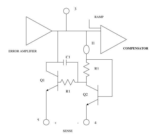
Since the gain of this circuit is relatively low, there is a transition region as the current limit amplifier takes over pulse width control from the error amplifier. For testing purposes threshold is defined as the input voltage required getting 25% duty cycle with the error amplifier signaling maximum duty cycle
