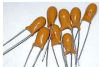
Solid-body, resin-dipped 10 \mu F 35 V Tantalum capacitors.
