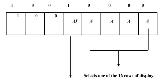
Auto increment = 1, the row address selected will be incremented after each of read and write operation of the display RAM.
